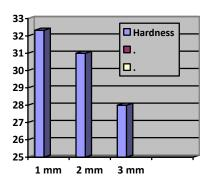
Effect of groove opening on weld bead hardness shown by graph below
